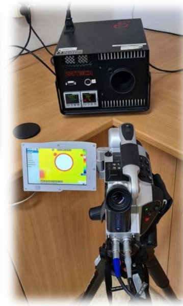
VarioCAM HD thermal camera with microscope lens - resolution \sim 35\mu\text{m}
