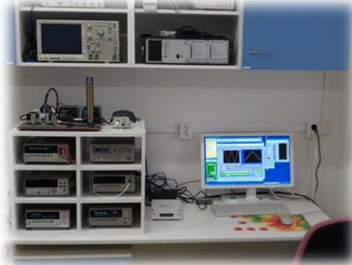
In-house developed systems for measurement of sensor properties, Electrometer Keithley 6517A and Keysight 34465A - precise measurement of high resistance materials with in-house fixtures with triaxial interconnection
