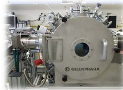
HV - Deposition system combining molecular evaporator (Creaphys DE-FR/2.2), thermal boat evaporator and pulsed laser deposition
